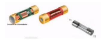
This fuse unit is in the form of a cartridge. It's normally manufactured in the range of 2A to 100A. Whenever the fuse blows off, fuse with carrier is replaced by a new one. As it is sealed, it cannot be rewired.
