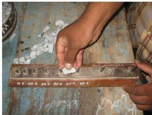
Elongation Index Test in Progress
