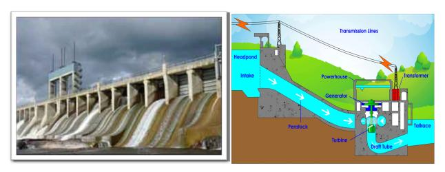
In **hydro power plant** we use gravitational force of fluid water to run the turbine which is coupled with electric generator to produce electricity. This power plant plays an important role to protect our fossil fuel which is limited, because the generated electricity in hydro power station is the use of water which is renewable source of energy and available in lots of amount without any cost.
