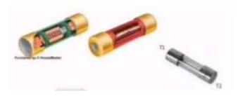
This fuse unit is in the form of a cartridge. It's normally manufactured in the range of 2A to 100A. Whenever the fuse blows off, fuse with carrier is replaced by a new one. As it is sealed, it cannot be rewired.
